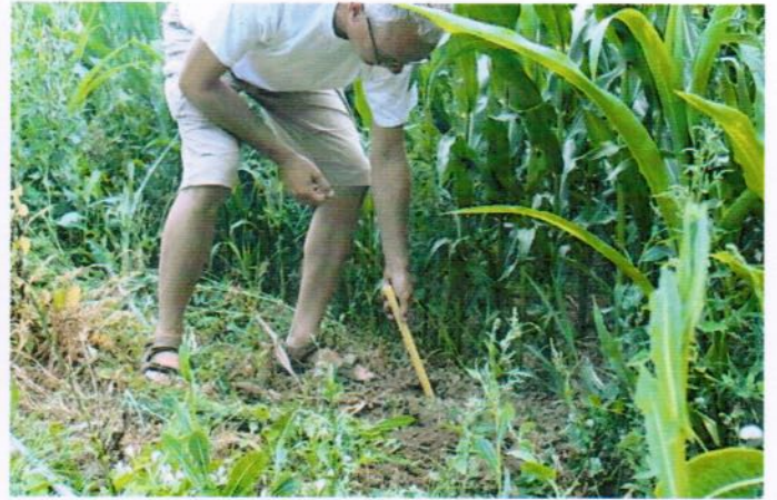
Place the guide pipe (ivory) into the hole
