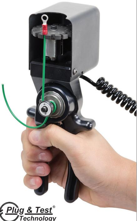
The MR06-200 wire crimp pull sensor is a hand-operated solution for measuring wire crimp pull-off forces. The ergonomic handles and convenient tensioning mechanism make field measurements a breeze for applications up to 200 lbF (1,000 N). Squeeze the handles together to increase tension on the sample until a break occurs. The peak force is recorded by the indicator.
