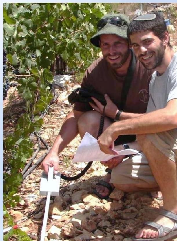
It was important to determine that LAI measurements were reliable and accurate and so in order to verify the accuracy of SunScan LAI measurements, leaves were removed from a total of eighteen 2m sections of grapevine and measured with an area meter.
