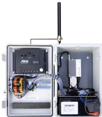
3G-DLC-BX1/SP modem gateway box (solar panel not shown)
