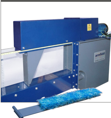
C4-67 - Wave generator and wave absorbing beach
