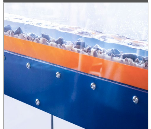
C4-69 - Artificially roughened bed
