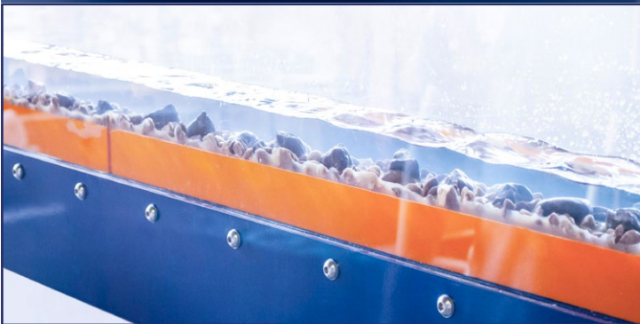
C4-69 - Artificially roughened bed
