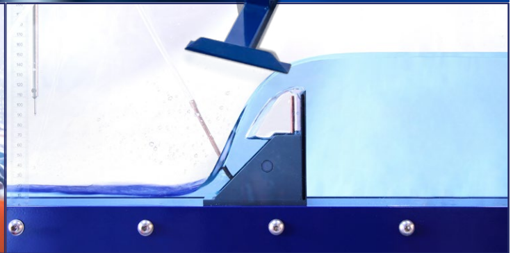
Sharp Crested Weir (in vented condition)
