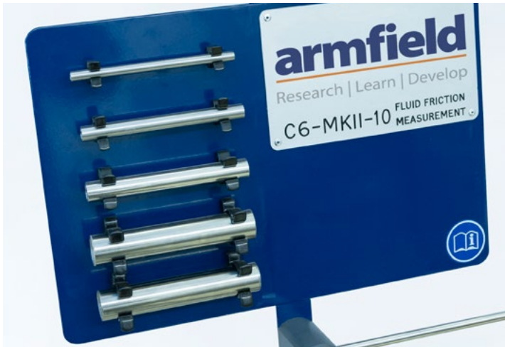
C6MKII Stainless steel pipe section and test pipe samples
