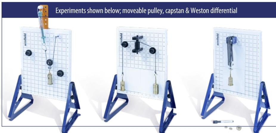
Experiments shown below; moveable pulley, capstan & Weston differential
