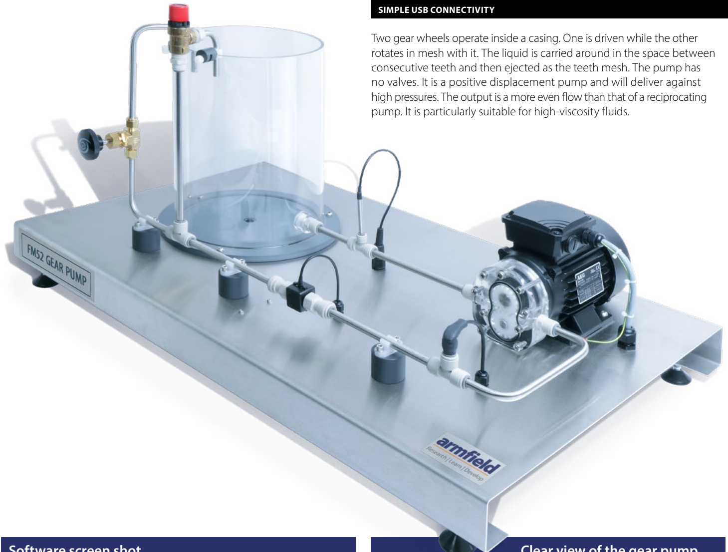
Clear view of the gear pump
