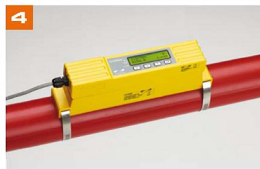
4 Click electronic assembly onto guide rail and sensor assembly
