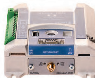
XLink 100 with exchangeable Iridium or Cellular modem card
