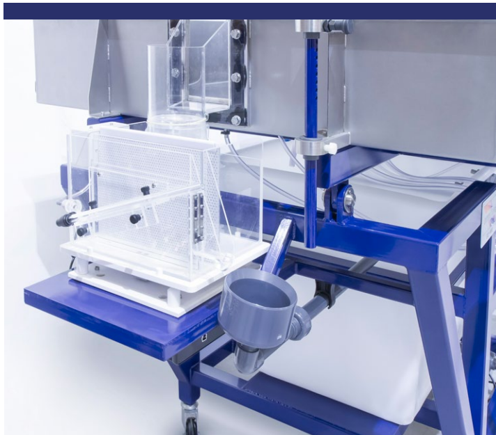
S12-MKII-50 - Inclined manometer for measuring of the height over the notch weir
