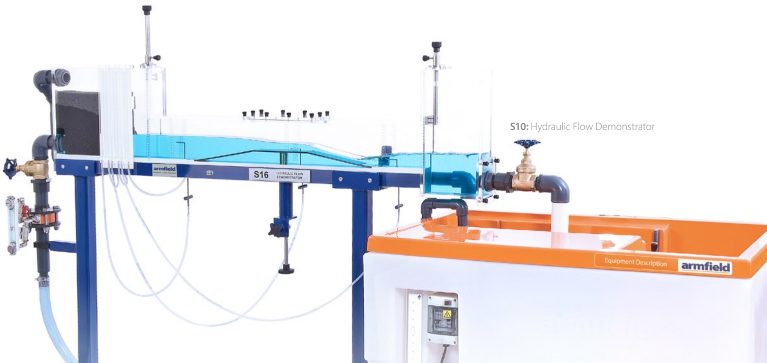
Unique elevating bed section and models of various hydraulic structures
