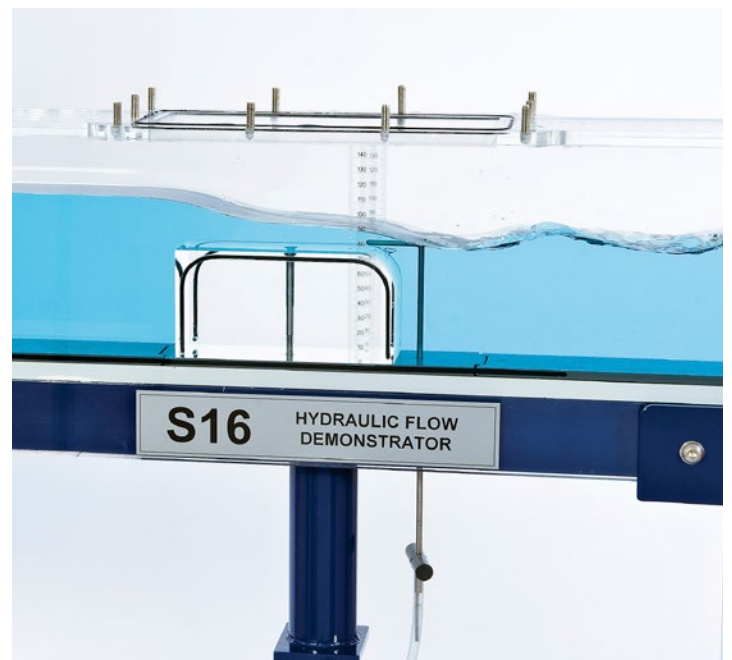
Surface oscillations downstream of a broad crested weir when the weir becomes drowned
