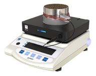
VARIOS generates thermal dryout curves automatically, so you can focus on other taksl. No manual process of getting the soil in and out of the oven. No repeated manual weighing of the sample. It's all taken care of for you, including data acquisition and analysis.
