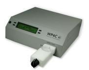
Fast, Accurate Water Potential Measurements - Use the WP4 to measure water potential in 5 to 10 minutes. Range: 0 to -300 MPa with a resolution of 0.1 MPa. The WP4 is a bench-top instrument with a lexan sample drawer. To make a reading, set a cup in the chamber and close and latch the drawer.
