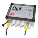
The DL6 is a dedicated data logger optimised for use with Delta-T soil moisture sensors. It can be used with combinations of ThetaProbes, SM150T Soil Moisture Sensors and Profile Probes, and also accepts rain gauge and soil temperature probe inputs. Up to 16000 readings can be stored in memory.
