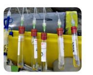
The standard Rhizon models have a diameter of 2.5 mm and a mean pore size of 0.15  $\mu$ m. They can be used for sampling pore water in pots, vessels or cylinders filled with settled soil, or directly in undisturbed cores.
