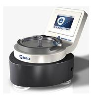
The Hosokawa Alpine Air Jet Sieve e200 LS has an attractive ergonomic design and fits nicely on a work bench. A high resolution 6.4"TFT touch screen allows intuitive operation with its easy-to-follow user interface.
