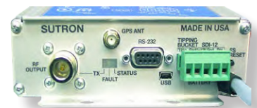
USB Mini Type B requires USB Type A Transition Cable. Sutron will provide 6 ft USB Cable upon request. Cable Part # 6411-1613.
