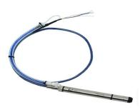
INW's patented PS9800 submersible pressure transmitter represents the latest in state-of-the-art level measurement technology. Building on years of successful experience, this industry standard two-wire, 4-20 mA device offers improved noise immunity, thermal performance and transient protection.
