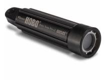
The HOBO Water Temp Pro v2 is durable with 12-bit resolution. Complete with a precision sensor for  $\pm 0.2^{\circ}$ C accuracy, this logger measures temperatures between -40°C and 70°C (-40°F to 158°F) in air and up to 50°C (122°F) in water. Its waterproof, streamlined case allows for extended deployment in fresh or salt water.
