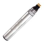
Cyclops-7F<sup>™</sup> Sensors are high performance, compact submersible sensors designed for integration into any platform that provides power and datalogging. Available with multiple optical configurations, Cyclops-7F Sensors have a universal I/O for connection to parent systems. Recently updated to have a faster settling time, Cyclops-7F is ready to make measurements 1 second after power up.
