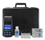
The DC1500 Chlorine Colorimeter Kit, ideal for both field and lab use, covers the entire critical chlorine range of 0-4 ppm with an MDL of 0.03 ppm. The Colorimeter is also EPA Compliant, (tablet version), using proper wavelength and DPD test method to meet EPA design specifications for NPDWR and NPDES chlorine monitoring programs (EPA 330.5 and Standard Method 4500).
