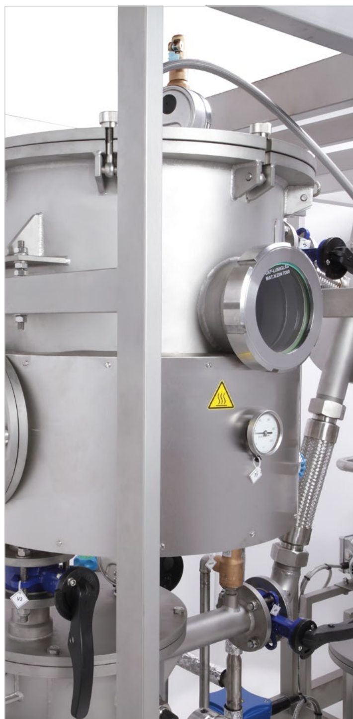
Desolventiser / extractor vessel with viewing port
