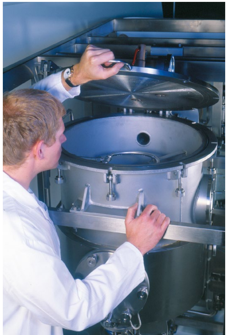
Inspecting the interior of the extractor vessel
