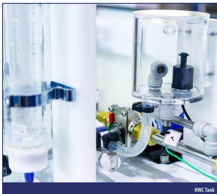
Reactor input / Output selector valve
