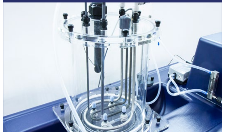
W11 digester detail
