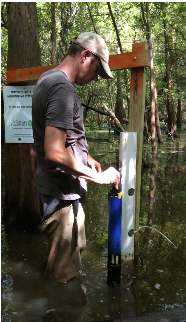
Joe Baustian of The Nature Conservancy deploys an EXO2 sonde in Louisiana's Atchafalaya Basin. Water quality data from the Conservancy's network of sondes is providing insight into the region's little-studied swamp forest.
