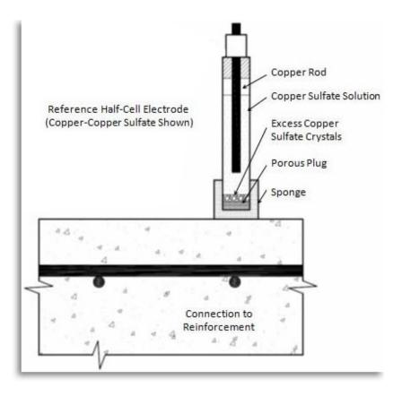
The reference electrode consists of a copper tube immersed in a copper sulfate solution. The surface electrical connection to the concrete is made through a solution-saturated sponge at the end of the probe. After the grounding connection to the rebar grid is made, the operator simply pushes the saturated sponge against the concrete to acquire a reading.
