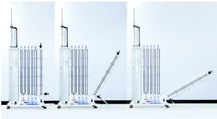
F1-29: Different inclination angles in the inclined manometer
