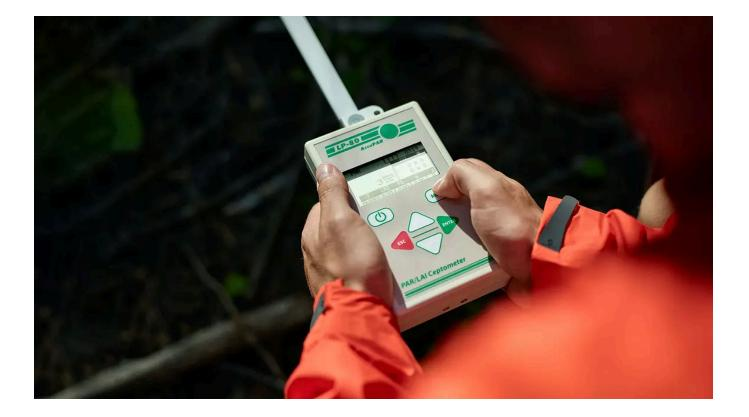
Looking for an alternative method, she discovered the LP-80 ceptometer: a lightweight, fieldportable instrument for measuring leaf area index. Using the LP-80, Zuckerman was able to rapidly assess the leaf area contribution of each tree species along the riparian corridor. Using this information, it was relatively straightforward for her to estimate the contribution of each tree species to the stream food web.
