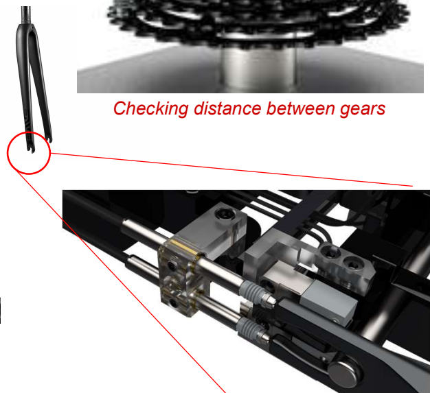
6mm probes and mini probes checking end of bicycle fork
