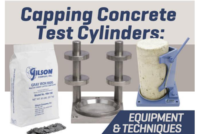
Testing concrete mixes delivered to a construction site ensures the quality and strength characteristics of the completed project. Representative sampling provides material for on-site temperature, consistency, and air content tests and casting of 4x8in or 6x12in concrete cylinders for laboratory compressive strength testing.
