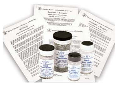
Sieve calibration with SRMs can be performed in-house by the user and avoids removing the sieves from service for shipping to a metrology lab. It can be a good choice when the actual opening dimensions of test sieves are critical.
