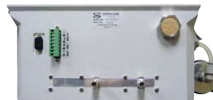
Dual Orifice Constant Flow Bubbler Connectors on Enclosure Bottom
