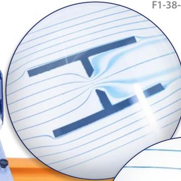
Sinks and sources may be used in combination with the flow of water between the plates to simulate a variety of flow situations.
