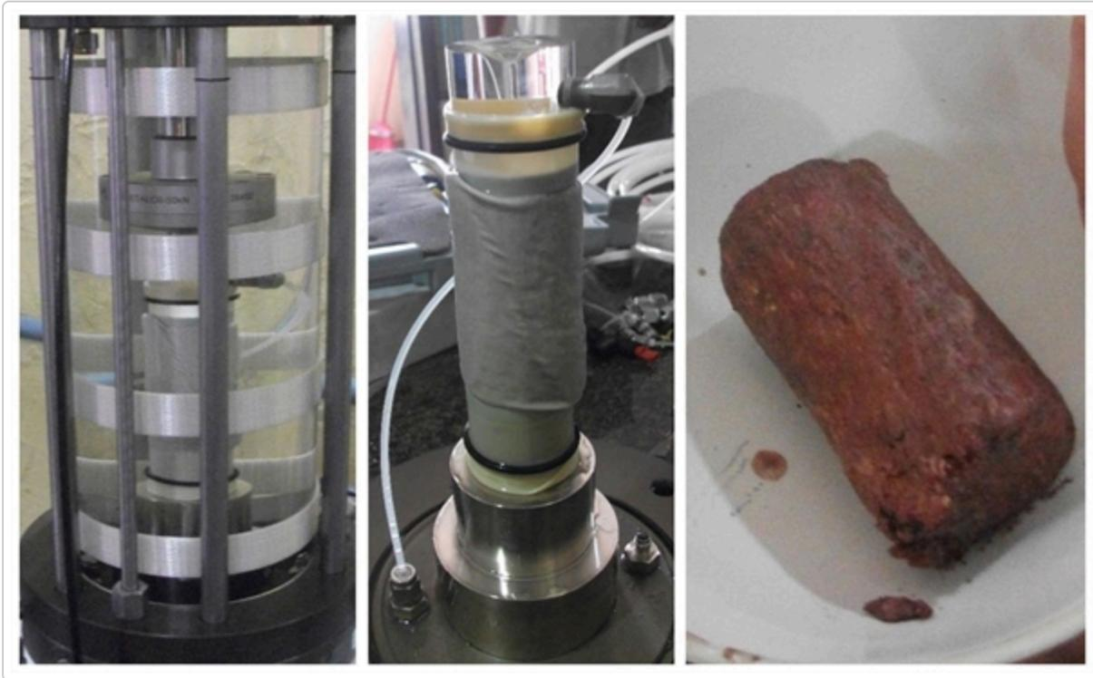
Figure 12: Photos of an isotropically-consolidated fine-grained soil specimen tested under undrained monotonic strain-controlled compression conditions within a GDSTAS. This test was in no way related to the Cadia NTSF embankment slump investigation, and is shown for illustrative purposes only.
