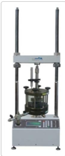
Figure 13: The GDS Constant Rate of Strain system (GDSCRS).
