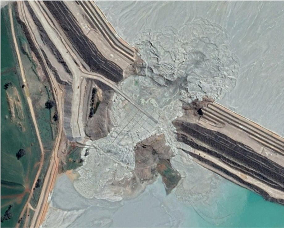
Figure 1: Aerial view of the Cadia NTSF southern embankment slump location as of the 13th of September 2018.
