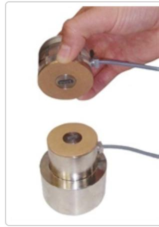
Figure 10: GDS Bender Element System (GDSBES).
