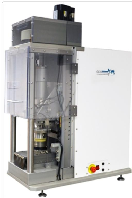
Figure 4: The GDS Electromechanical Dynamic Cyclic Simple Shear (EMDCSS) device.
