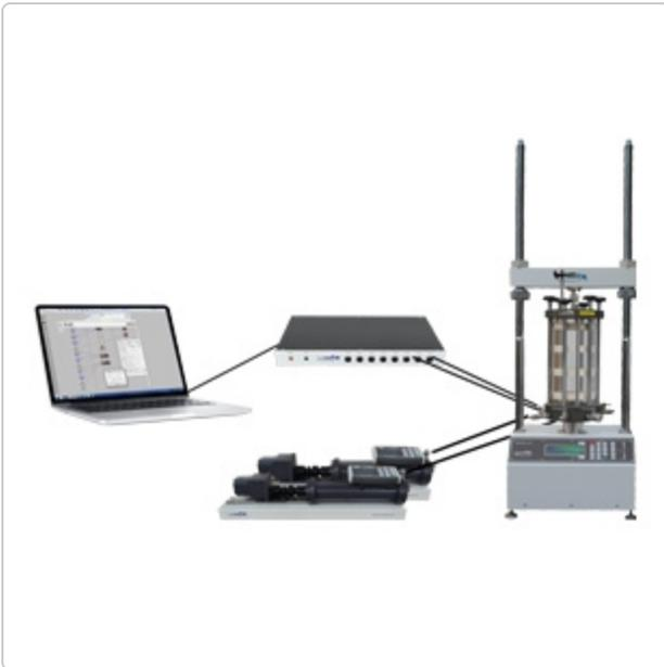
Figure 8: The GDS Triaxial Automated System (GDS TAS).
