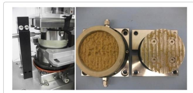
Figure 4: Cyclic direct simple shear response and photos of a clean sand specimen tested under
