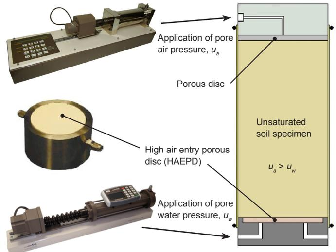
**Figure 8 – Typical unsaturated soil specimen set-up.**
