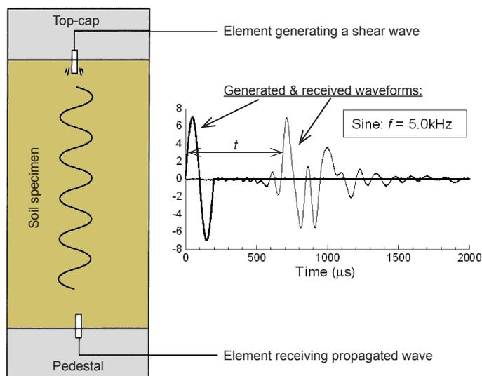
Figure 5 – Schematic illustration of an S-wave bender element test, displaying generated and received waveforms.
