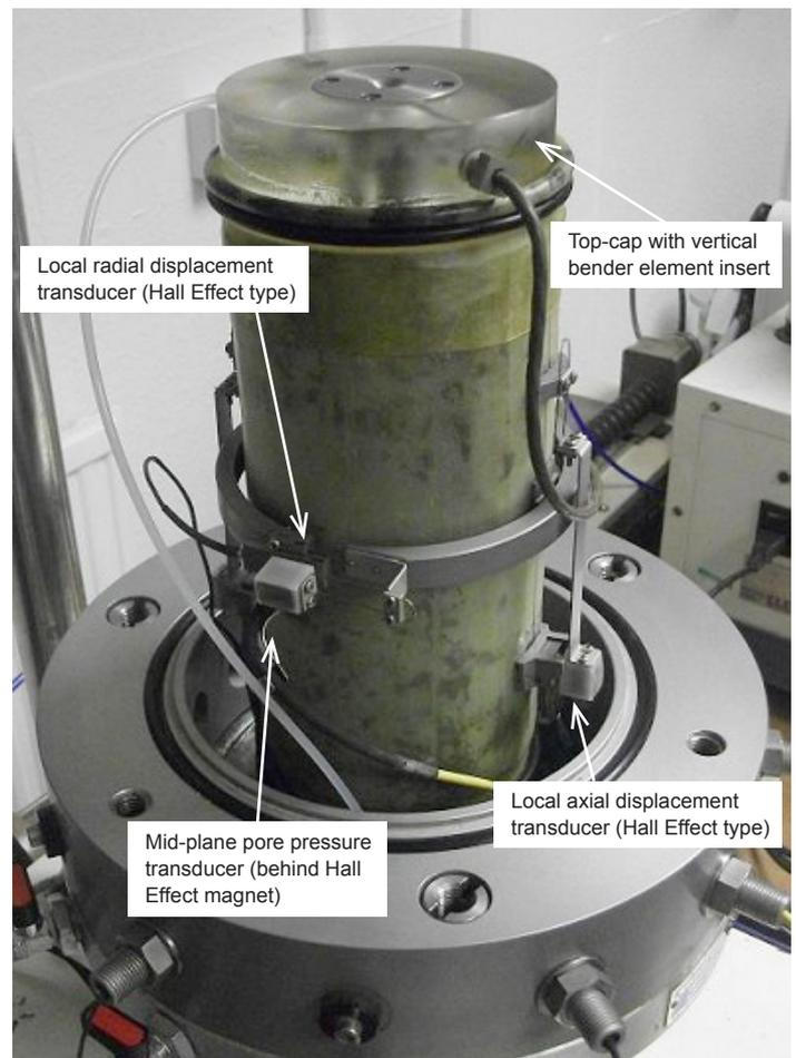
Figure 1 – Triaxial test specimen instrumented with local axial and radial Hall Effect transducers, mid-plane pore pressure transducer, and vertical bender elements.
