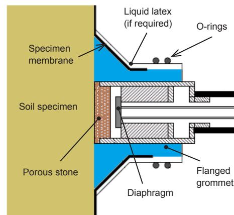
Figure 4 – Schematic illustration of a mid-plane pore pressure transducer mounted on a soil specimen (modified from Meilani et al., 2002).
