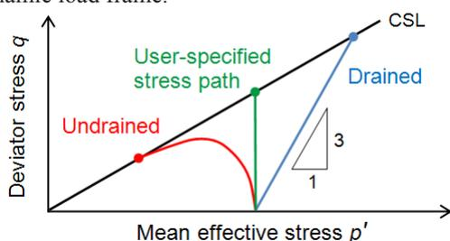
Figure 9 – Generalised stress paths for consolidated drained and undrained shearing, and a user-specified stress path in which the mean effective stress is held constant. Note all specimens are sheared to critical state, as defined by the critical state line, CSL.
