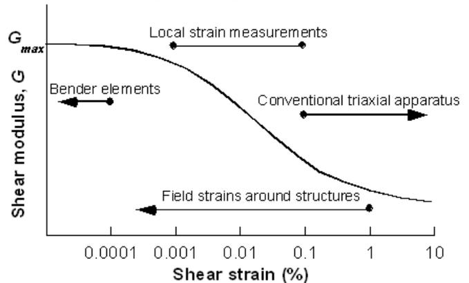
Figure 3 – Generalised shear modulus degradation curve displaying approximate obtainable strain ranges for various laboratory tests (modified from Menzies & Matthews, 1996).
