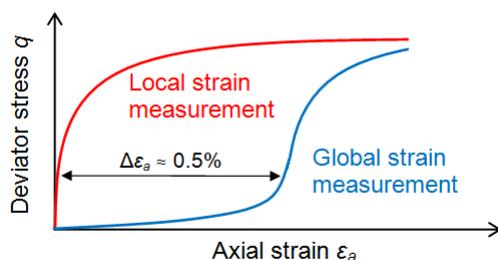
Figure 2 – Generalised specimen response during shear when taking both global and local axial strain measurements.
