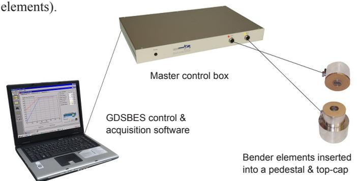
Figure 6 – GDS Bender Element System (BES) components.
