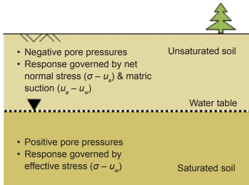
**Figure 7 – Simplified illustration of saturated and unsaturated soil mechanics.**
