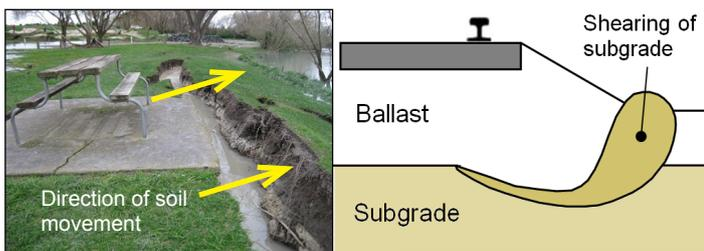
**Figure 1 – Earthquake-induced lateral spreading (left); illustration of progressive railway subgrade shear failure due to repeated load cycles (right, reproduced from Mott MacDonald, 2011).**
