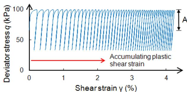
Figure 3 – Accumulation of plastic shear strain during an undrained cyclic loading test on a sand specimen.
