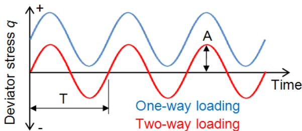
Figure 2 – One-way and two-way cyclic loading patterns. Note  $T$  = loading period and  $A$  = loading amplitude.
