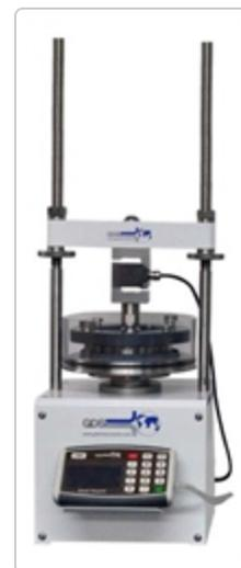
Figure 7: GDS Automatic Oedometer System (GDSAOS).
