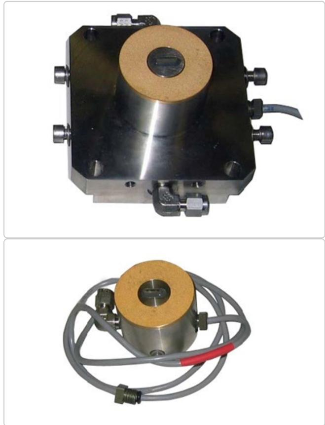
Figure: 5 Bender Element shown in pedestal and topcap.
