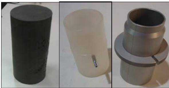
Figure 5 – Trimmed cohesive specimen (left); membrane suction stretcher (middle); split-part mould for granular specimen preparation (right).
