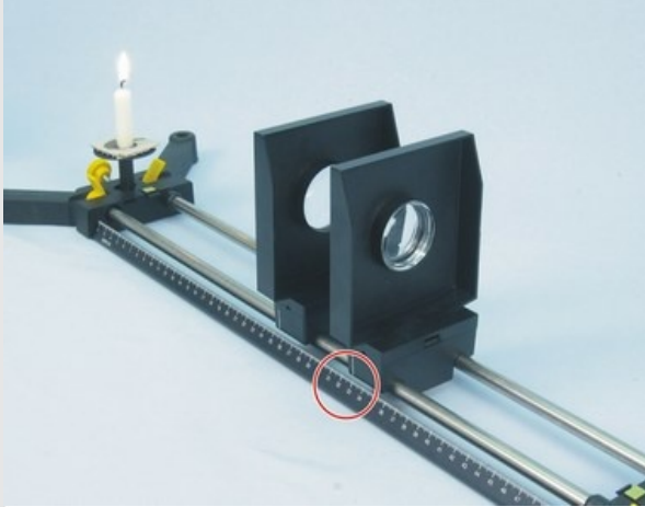
Measurement of the distance between the two lenses
