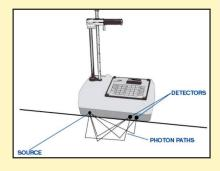
This is a rapid, nondestructive means of testing materials (usually asphalt and concrete) that are approximately 4 in (10 cm) in depth. The gamma source remains inside the gauge, and the gamma rays that are scattered back toward the detectors are counted to determine the density.
