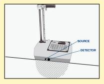
Moisture content is measured in a nondestructive test mode. Moisture is determined through the detection of thermalized neutrons (i.e., "fast" neutrons that have been slowed by the hydrogen present in the material [normally in the form of water]).
