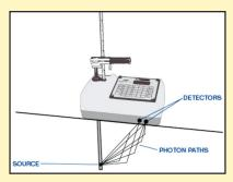
The source rod extends through the base of the gauge into a predrilled hole up to 12 in (30 cm) deep in the material being tested. Gamma rays are transmitted from the density source through the test material and counted by detectors located within the gauge.
