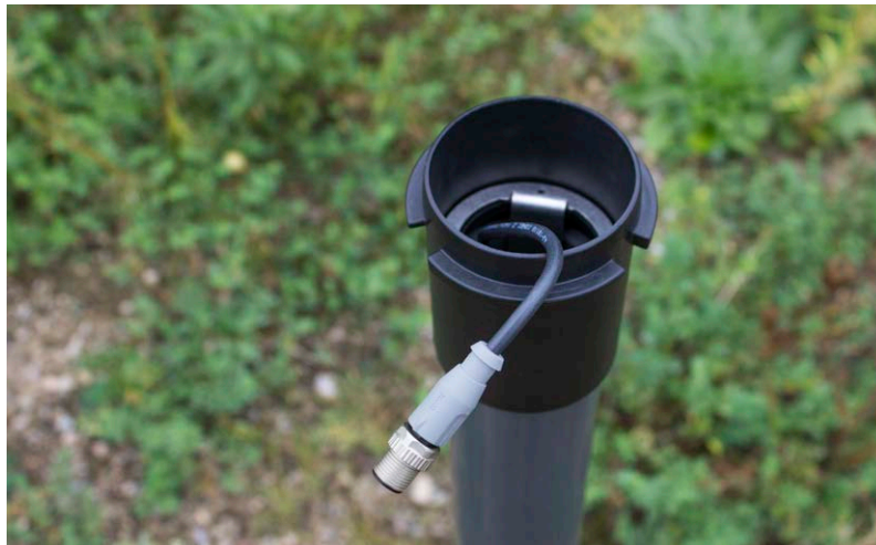
Figure 6-6 Lower the Assembly into the Well
