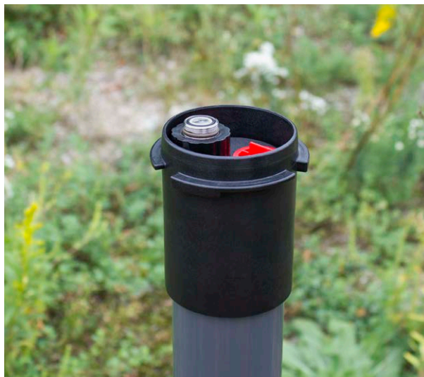
Remove Existing Levellogger Installation
