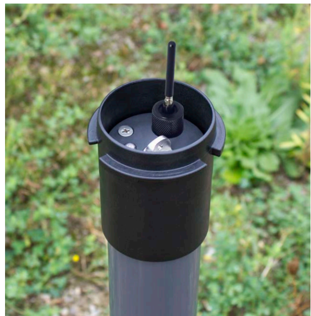
Figure 6-8 Lower the LevelSender into Position
