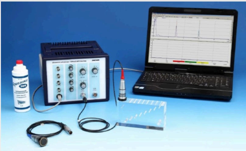
Fig. 1: Equipment for ultrasonic echography, experimental set-up
