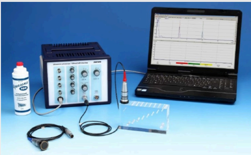
Fig. 1: Equipment for ultrasonic echography, experimental set-up
