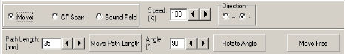
Fig. 3: Software: parameters for moving the scanner
