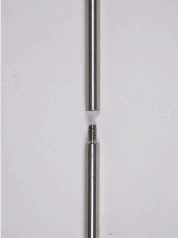
Screwing the support rods
