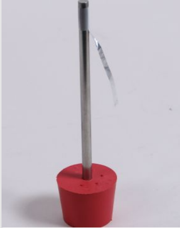
Attach the guide foil strip to the stand rod
