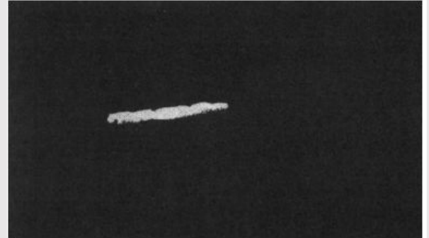
Fig. 6: Track generated by an \alpha -particle.
