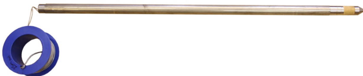
Fig. 1 – The piezometer is available in several versions – with or without logging function. Pressure transducer, A/D converter, processor with optional log memory and battery are integrated in the probe. Only the cable is visible on the surface.
