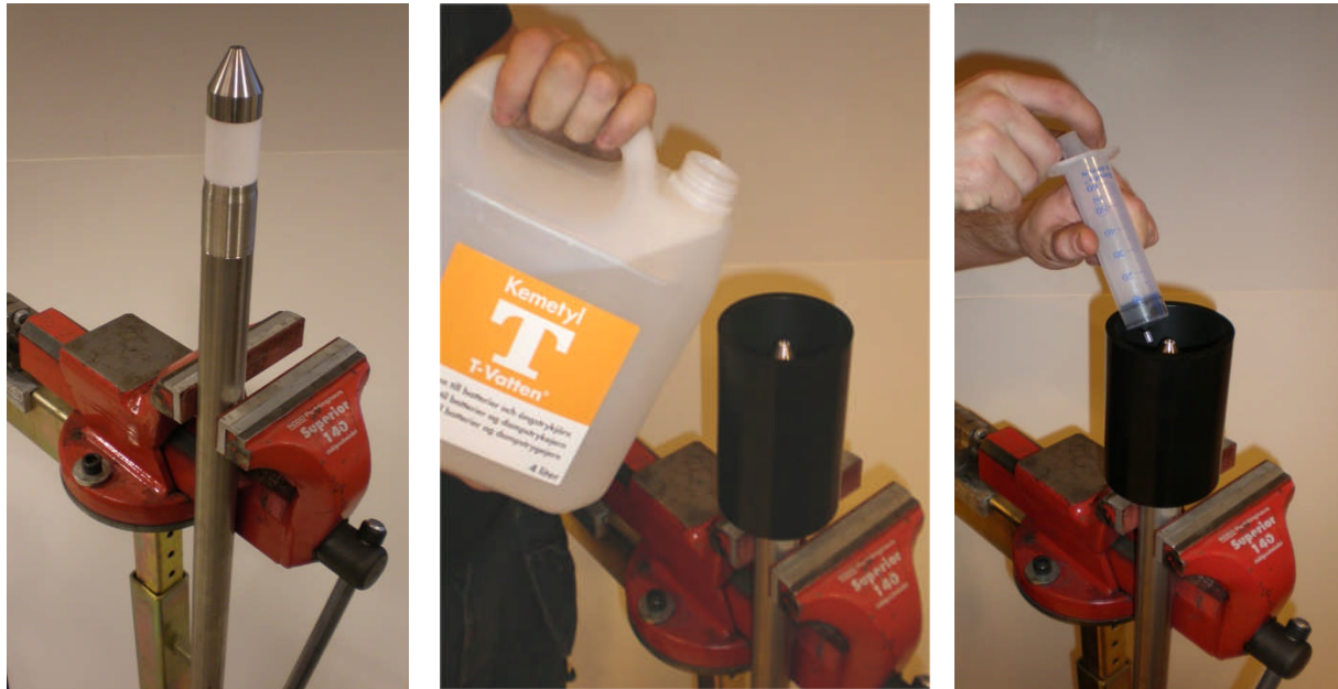
Fig. 7 – Keep the filter of the de-aired probe under water.
