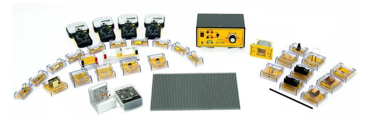
The kit is composed of a set of components and devices that allow a practical demonstration of the most important laws of electricity and electromagnetism.
