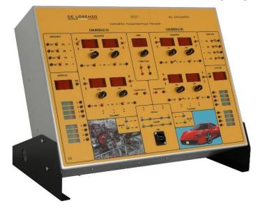
The system has been designed for the study of electronic systems with can bus architecture, based on CAN OPEN protocols.
