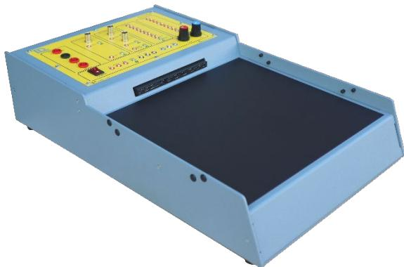
Power supply unit for the TIME boards system with virtual instrumentation. It includes an interface board to insert faults from the management software and dedicated inputs and outputs for the virtual instruments.
