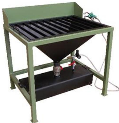
Machine for impregnating in a simple and clean way the electric motors.
