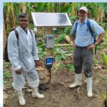
Professor Jerry Knox works and colleague installing Delta-T sensors and loggers
