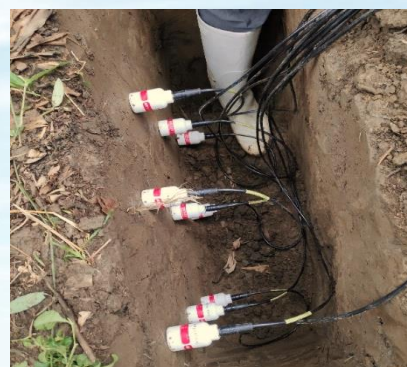
Professor Jerry Knox works and colleague installing Delta-T sensors and loggers
