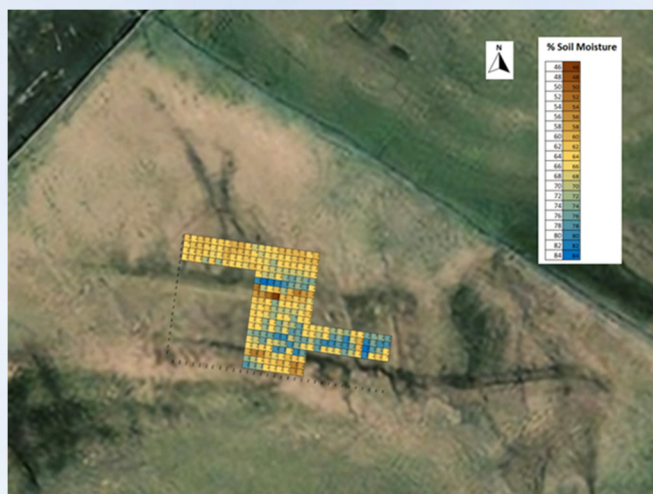
Pic a. Soil moisture grid measurements on Widdybank Meadow.
