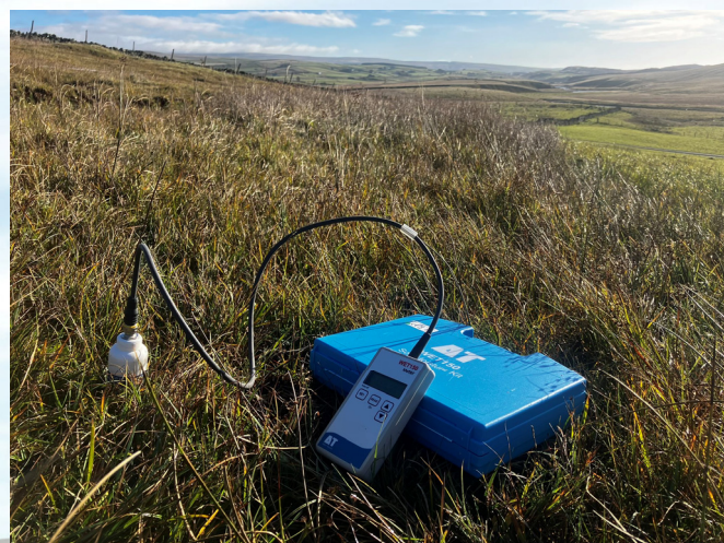
The portable Wet150 Sensor and readout meter kit used at Widdybank Fell.
