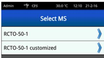
After attaching any measuring system to the instrument, the automated spindle-detection will recognize the type (e.g. RCTO-50-1) and the serial number of this spindle. This settings menu provides the possibility to customize the parameters of the detected spindle. For best accuracy, it is recommended to enter the parameters from the spindle protocol and an appropriate name.
